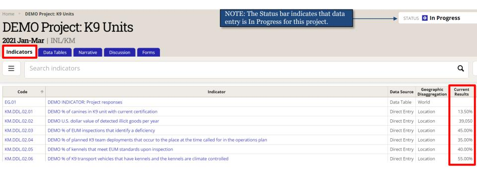
NOTE: Each time you return to the **Indicators** tab, you will see data entry for each indicator summarized and reflected in the "Current Results" column. Although this is a good way to track the indicators for which you've begun entering data, note that these totals do not denote entry completeness. Users must click into each indicator in order to confirm the accuracy and completeness of their data entry!
